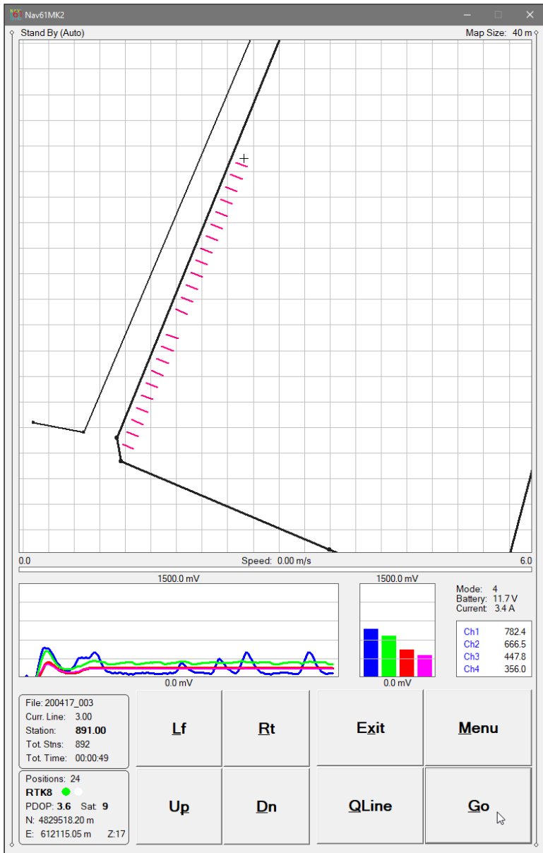
Figure 8.59: Nav61MK2 portrait orientation - Stand By mode, two background user files displayed, positions shown as swath bar.
