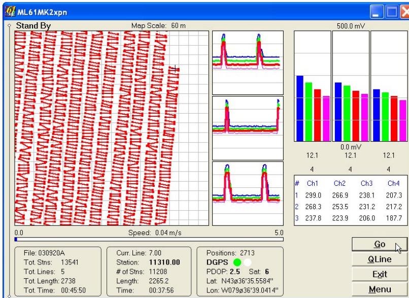
Figure 1.11 ML61MK2xpn screen in Navigation mode, Swath Bars represent positions of a three units array (3 m width) on a 60 m scale map.
