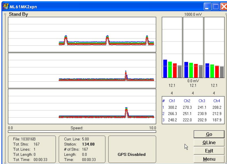
Figure 9.29: ML61MK2xpn Screen in Stand By mode after Readings Scale change, compare with Figure 9.28
